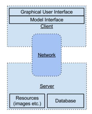
The drawing explains the basic concept of the system with three major subsystems and how they're interconnected. It also shows the different layers make up the client.
